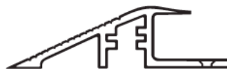
Aluminum ramping (for 14mm height grid only, with screws & rawl plugs supplied)
